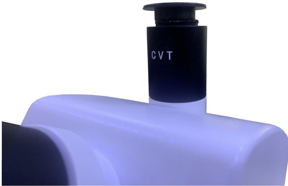
Figure 7 CVT adapter (top of device)
